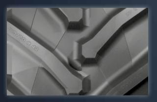
The **inter-lug terracing** is an advanced design at the base of the lug which helps with mud ejection, maximizing the selfcleaning capability of the tire.
