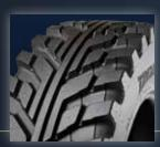
The progressive widening of lugs towards the shoulder, and the distinctive terraces design, increase self-cleaning and traction.
