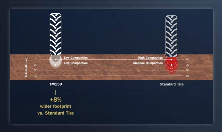
As you go deeper into the soil, the standard tire causes compaction that worsens rapidly. At 20cm depth, the TM150 maintains "low" compaction, while the standard tire is already experiencing "medium" compaction.
