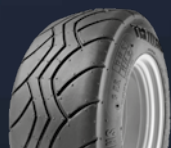
Green area tire for professional haymaking machinery with high stubble resistance.
