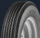
High Speed tire with high shoulder.
